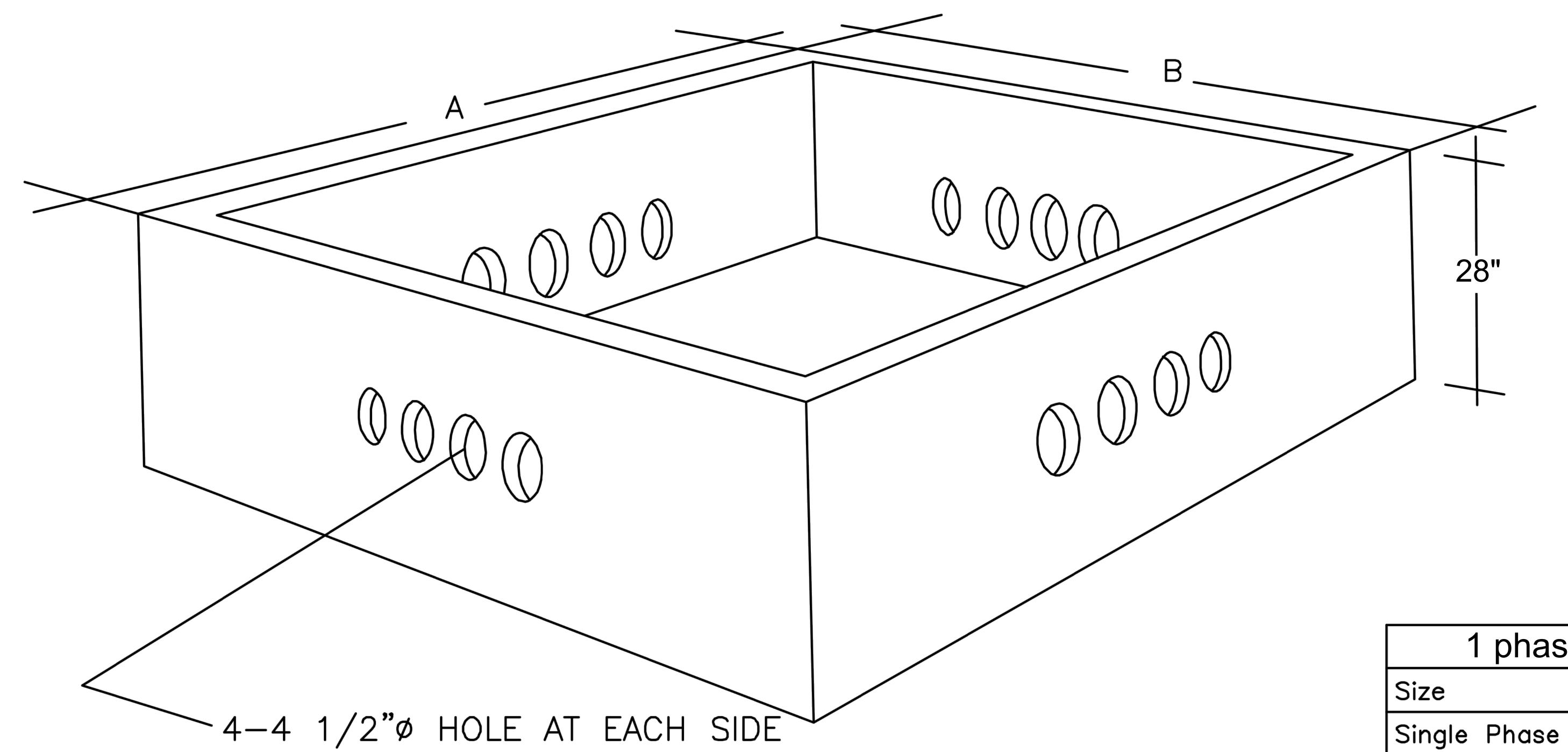
4" THICK PRECAST REINFORCED CONCRETE WITH 6X6 6/6 W.W.M. OR #3 REBARS SPACED @ 12" O.C. B.W.
